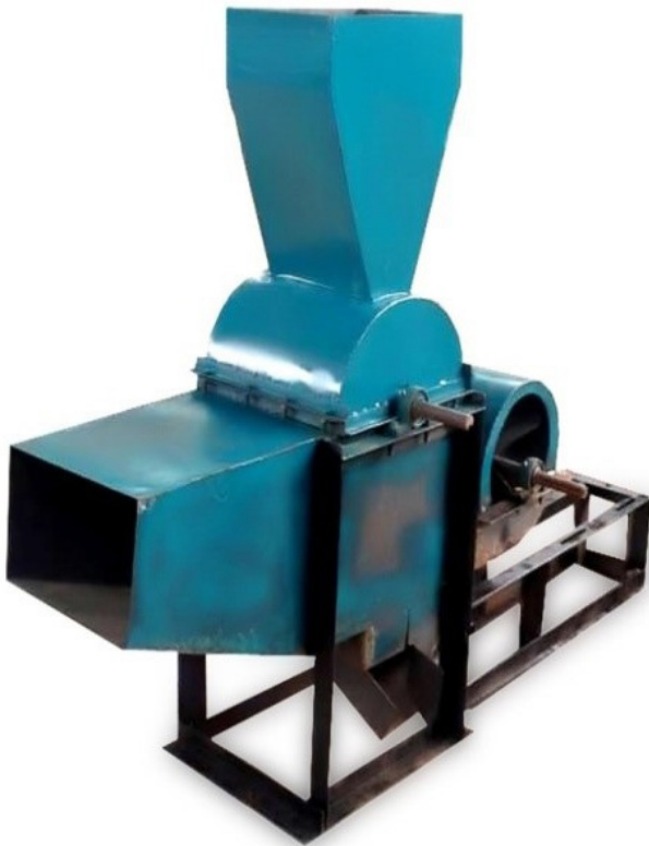
Figure 4: Fabricated Jatropha curcas seed sheller
